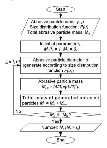
Fig. 4. Schematic of the calculation of abrasive particle number at each dwell position.
