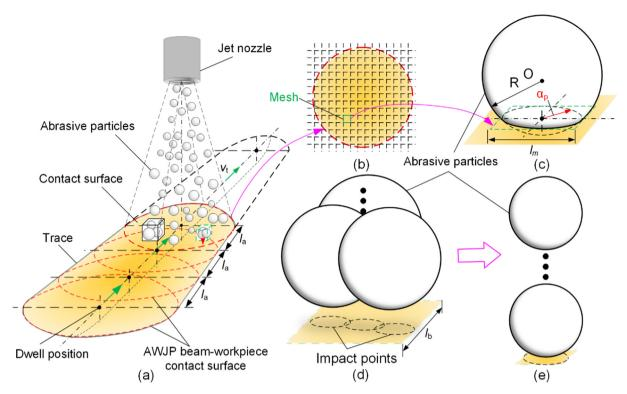
**Fig. 3.** Schematics of abrasive particle–workpiece contact and superposition process. (a) Peening process of a single trace, (b) division of contact area between abrasive waterjet beam and workpiece at dwell position, (c) mesh size setting process, (d) number of abrasive particles in each mesh, and (e) overlapping approximation of abrasive particles impact within the same mesh.
