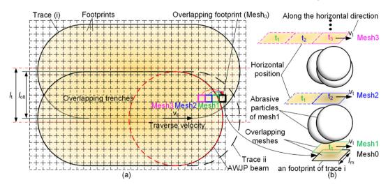
Fig. 5. Schematics of footprint superposition analysis process of traces with overlapping process of (a) two adjacent traces and (b) meshes (jet beam at different dwell position).
