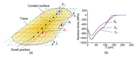
Fig. 7. Schematics of (a) equivalent load distribution and (b) corresponding residual stress.
