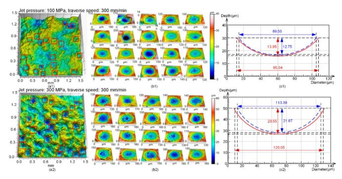
**Fig. 12.** Schematics of footprints of multiple abrasive particles and a single abrasive particle footprint. (a1, a2) Experimental footprint with traverse speed 300 mm/min and jet pressures of 100 and 300 MPa, respectively, (b1, b2) abrasive particle footprint of special position in (a1) and (a2), (c1, c2) mean footprints depth and abrasive-workpiece contact diameter of 20 abrasive particles footprints in (b1) and (b2) and the corresponding calculated values according to the modelling.
