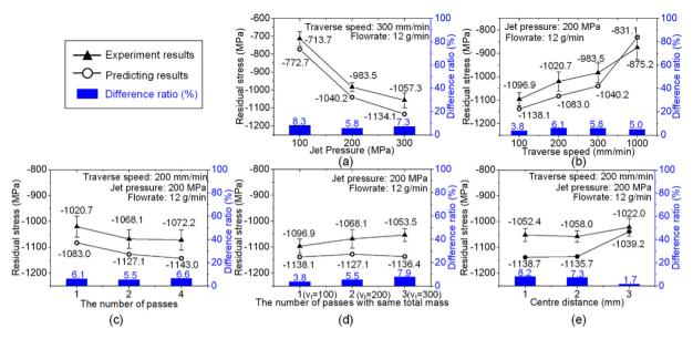
**Fig. 15.** Comparison of predicting and experimental maximum compressive residual stresses, and the varying trend of the maximum compressive residual stress with different peening parameters. a) Jet pressure, b) traverse speed, c) number of peening with different abrasive mass, d) number of peening with the same abrasive mass, and e) centre distance effect on compressive residual stress.
