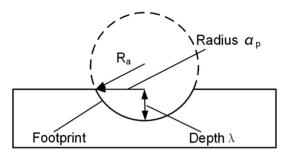
Fig. 10. Schematics of the abrasive particle radius calculated process.
