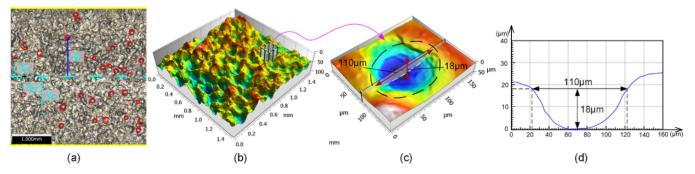
**Fig. 9.** Schematics of data collection process. (a) experimental surface topography with pump pressure 200 MPa, abrasive flow rate 12 g/min, traverse speed 1000 mm/min, (b) 3D graph of mountain map software at dwell position, (c, d) measurement of footprint depth with 3D and 2D topography, respectively.
