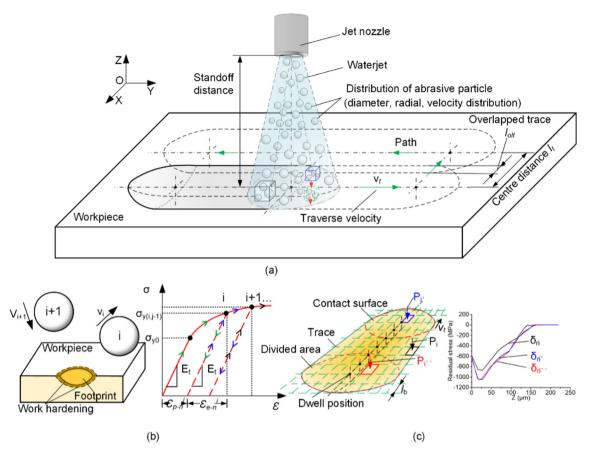
Fig. 1. Schematics of AWJP process: with (a) abrasive particle size, spatial, velocity distribution in waterjet, and overlapped traces; (b) work hardening between two impacted abrasive particles; and (c) distribution of equivalent load and corresponding compressive residual stress.
