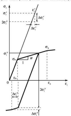
$\textbf{Fig. A1.} \ \ \textbf{Stress-strain} \ \ \textbf{relationship} \ \ \textbf{of} \ \ \textbf{the} \ \ \textbf{loading} \ \ \textbf{and} \ \ \textbf{unloading} \ \ \textbf{process}.$
