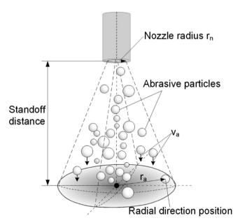
Fig. 2. Schematic of abrasive particles distribution within the waterjet beam.
